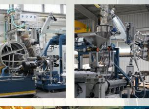
Today, a single machine can produce pipes with diameters ranging from DN/ID 400 to DN/ID 3500, lengths of up to 6 meters, and a variety of stiffnesses, pressure classes, and profile options.
