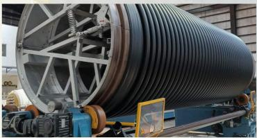
A profile is being extruded by an extruder or compounder. This heated profile is helical wound on a turning and foldable mandrel. Without using any welding, the heated profile, which may be either a solid or structured wall, is melted together. The mandrel size determines the pipe diameter, so the pipe is always measured by its inside diameter. The pipe wall is always completely homogeneous, and the inner surface is very smooth.
